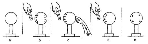
3. The diagrams below show a similar procedure with a positive rod. Draw the correct charges in diagrams (a) through (e).
